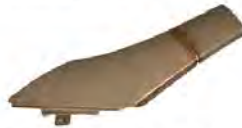
Robot coldArc brazing, 1.0 mm electrolytic zinc-plating steel panel, 1.0 mm CuSi3 wire
