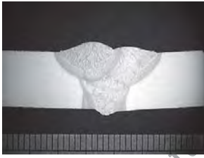
A 5-pass single wire 10mm butt weld
