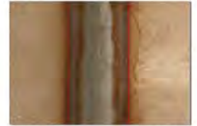
Only after welding 3 layers of forceArc do we achieve the equivalent inter-run temperature of 2 layers of standard spray arc.
