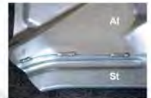
coldArc fusion of aluminium/steel mixed connections with zinc-based wire
