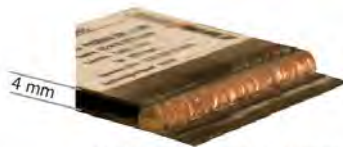
Manual coldArc-brazing, 4.0 mm gap 1.0 mm DC 04 ZE 75/75, 1.0 mm CuSi3 wire
