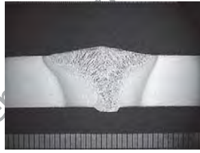
A 2-pass tandem wire 10mm butt weld
