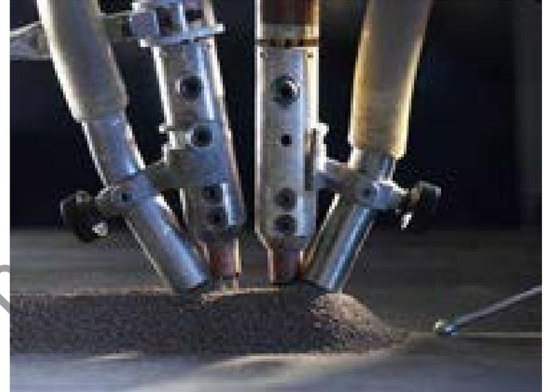
High efficient Submerged arc welding techniques
