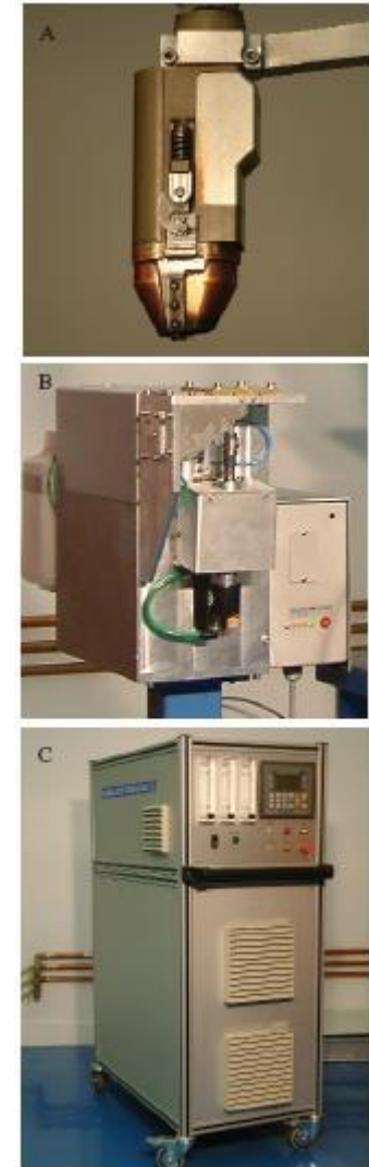
Fig. 2 — System components. A — Torch; B — cleaning station; C — interface.
