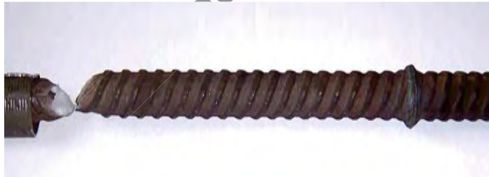
Pull test of weld joint of Reinforcement Rod - OD 32 mm
