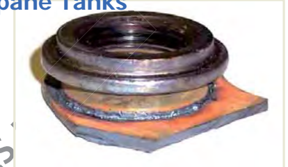
LP Tank Assembly, Boss Weld Size: OD 31.7 mm, WT 4.1 mm Welding Time: 7 Second
