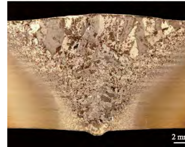
Macrographs of keyhole GTA welds in 13 mm thick ASTM B265 Grade 5-95a (Ti-6Al-4V) plate. The upper photo shows a single pass keyhole GTA weld while the lower has an additional dressing pass for improved bead profile.
