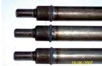
Piston Assembly: OD22x2.2mm Welding Time: 3.6 s
