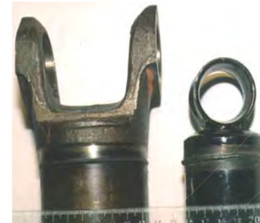
Shock absorber Welded section: OD53x1,8mm. Productivity: 200 butts/hour Welding time: t=2.9 s Material: Steel 20 + Steel 35
