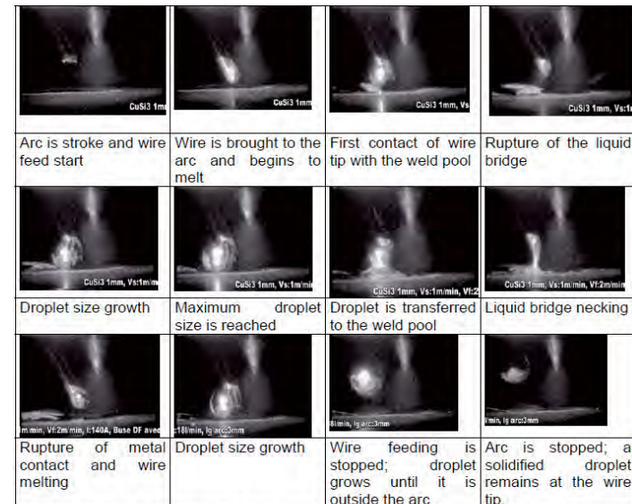
Figure 5 Droplet metal transfer mode during one complete welding cycle Galvanized steel, \varnothing 1 mm (0.040") CuSi3 wire I=140 A, WFS=2 m/min (79 in/min), TS=1 m/min (40 in/min), t=3 mm (1/8")
