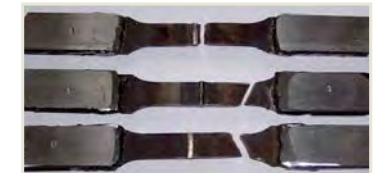
Welded Joint after Tensile Elongation Test
