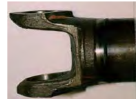
Drive Shaft OD75x2.1 mm Welding time: 3.8 s
