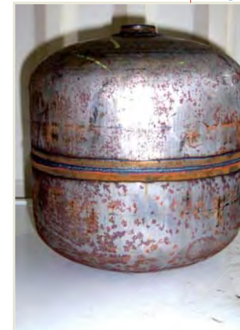
LP Tank Assembly, Girth Weld Size: OD203.2, WT2.1 mm Welding Time: 12.5 s
