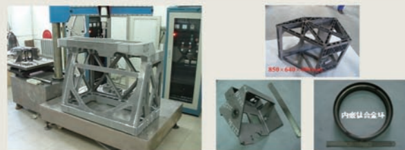
典型铝基复合材料超声波辅助钎焊构件 Typical ultrasonically soldered components of AlMMCs
