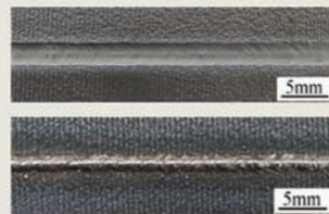
Ti600电子束焊接接头成形 Appearance of Ti600 electron beam welding joints
