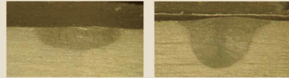
5mm厚304不锈钢TIG和A-TIG焊对比 Cross Sections of A-TIG VS TIGwelding: (a) TIG (b) A-TIG
