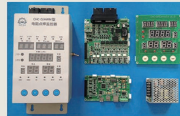
车身电阻点焊过程稳定性评价装置产品 Products of RSW monitors for Auto-body
