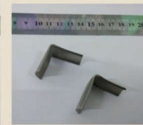
钛-不锈钢复合过渡接头管拉伸及弯曲试验结果 Tensile and bending test results of titanium-stainless steel transition joint tube
