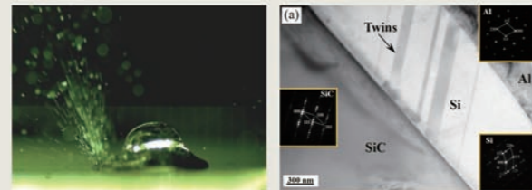
超声波激励作用下液态钎料的铺展与界面结合特征 Solder spreading and interface bonding under ultrasonication
