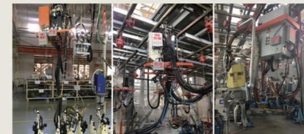
车身电阻点焊过程稳定性评价装置在整车厂的应用 Application of RSW monitors in Auto-manufacturing
