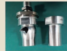
钛-不锈钢复合过渡接头管胀破试验结果 Bulge test result of titanium-stainless steel transition joint tube
