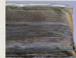
不锈钢墙体结构沉积体 Deposition of wall structure for stainless steel
