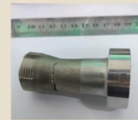
钛-不锈钢复合过渡接头管拉伸及弯曲试验结果 Tensile and bending test results of titanium-stainless steel transition joint tube
