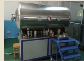
离子注入与沉积工业化装备 Ion implantation equipment
